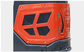
6 balance weight The rear part is equipped with a cast iron counterweight, which improves the digging balance of the excavator.
