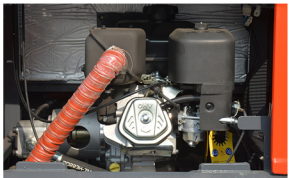
3 Flip-up rear cover on the seat The rear cover close to the seat opens wide, facilitating daily inspection of the engine and fuel system as well as parts replacement.
