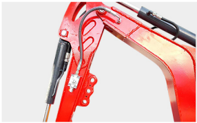
7 Strong forearms Built-in tubing, more beautiful, prevents tubing from wind and sun, increases tubing life, built-in explosion-proof steelwire.
