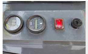
2 dashboard The operation box is equipped with instruments, which can monitor the excavator's status in real time.
