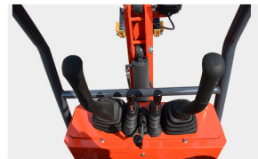
1 Front-mounted control lever The front-mounted operating lever ensures ample space for the feet and around the driver's seat.
