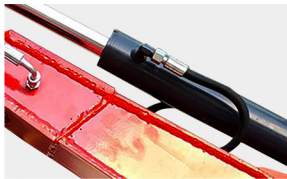
8 stamping cylinder One-piece stamping cylinder with enlarged cylinder diameter and imported oil seal is not easy to break and has longer service life.
