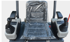
1 both sides control lever The both sides operating lever ensures ample space for the feet and around the driver's seat.
